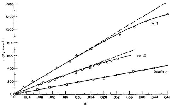
FIG. 4. Stress-strain curves of iron and quartz:
