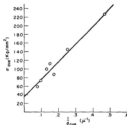
FIG. 10. The average strength of copper whiskers as a function of the reciprocal of the diameter.
