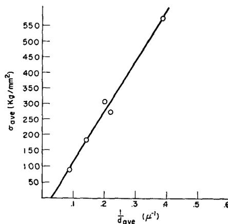
FIG. 9. The average strength of iron whiskers as a function of the reciprocal of the diameter.
